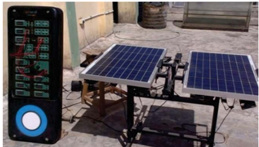
Figure 2: Solar PV Training and Research Kit
